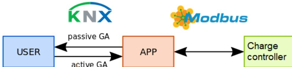
Since the connection via Modbus TCP compared to the pure data transmission requires significant time, the P-Charge APP reads the complete memory dump of the charge controller on demand or after a set period of time and sends the information to programmable KNX group addresses. If writable registers are to be changed via KNX, this is executed immediately.
